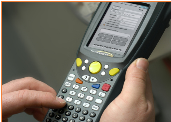
Figure 3. Software on the handheld PC to manage inspection schedules for each asset, capture inspection results in the field (as seen below) and track assets through the on-hire/off-hire process
