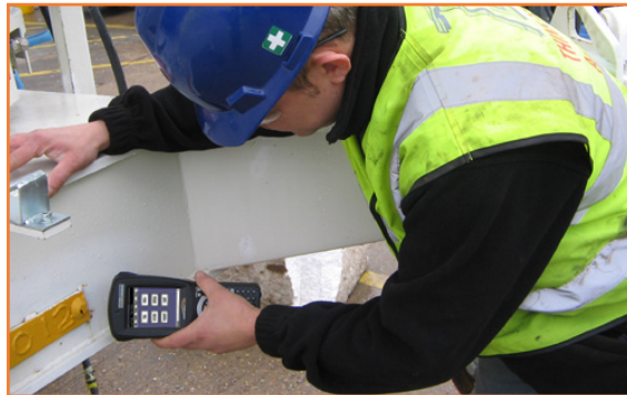
Figure 2. Tagged assets can be instantly scanned and identified using handheld PCs
